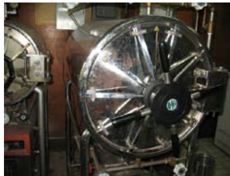
Autoclave used for sterilizing reusable medical equipments and other medical and laboratory supplies.
